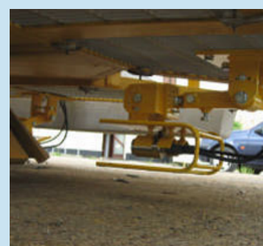
Brackets positioning the cameras a) Camera 4 witnessing the hydraulic locking pin and b) Camera 2 beneath the structure
